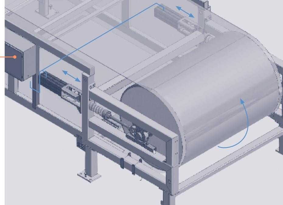
Pulley head frame with belt tensioning and tracking system.
