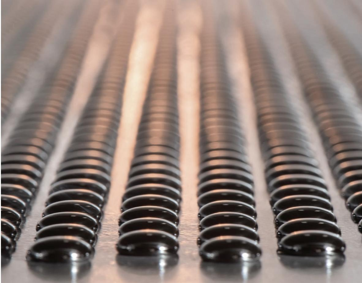
The highly uniform shape, stability and quality of Rotoform bitumen pastilles makes them ideal for packaging, storage, blending and further processing.
