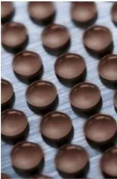
It solidifies these subcooling melts by introducing a homogeneous suspension of crystal nuclei into the melt. This enables the slurry (a mix of nuclei and liquid product) to crystallize quickly on the water-cooled steel belt of the Rotoform unit.
