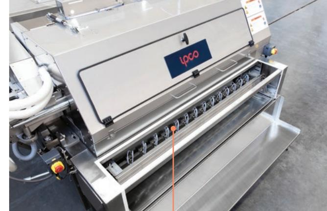
Spraying bar with nozzles.
