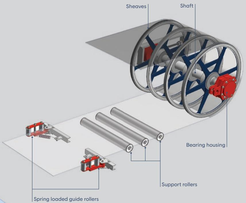
\* This illustration shows all types of IPCO conveyor components mounted on a single conveyor. Actual applications will vary.
