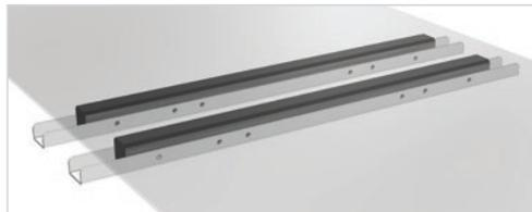
To ensure the best working conditions for carbon steel belts, we recommend that graphite be deposited on the underside of the belt at regular intervals between cast iron supports. IPCO graphite skid bars are designed to leave a deposit of lubricating graphite on the underside of the belt in a continuous and automatic way, and have the added benefit of providing lower friction than cast iron supports.
