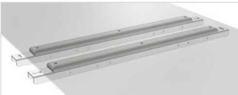
The iron in IPCO's cast iron skid bars is specially formulated and manufactured to provide optimal performance with carbon steel belts. Additionally, the surface of each skid bar is machine finished to provide a surface roughness of no more than Ramax=3.0  $\mu\text{m}$ .
