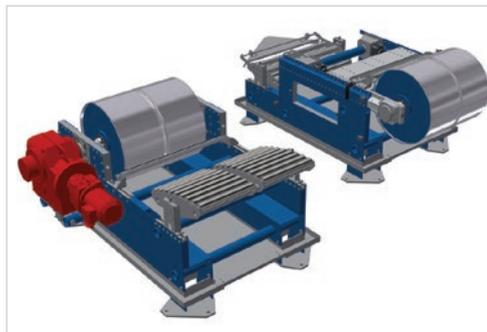
The end stations are the most complex part of a conveyor. Besides providing a sturdy 'anchor' from which to keep the pulleys in position, end stations must also allow for accurate tensioning of the belt and for providing motive power to the belt. Conveyor and process accessories are often placed at the ends stations as well, complicating them further.
