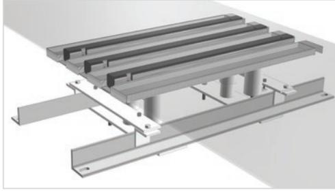
The IPCO graphite station is a standardized solution for depositing graphite on the underside of the belt. In bake ovens or in applications where the belt is cooled with water it can prevent oxidation. Installed close to the terminal drums it offers easy access for inspection and service.
